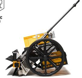
Basic function Hand-guided fruit harvester with electrically driven collecting roller
