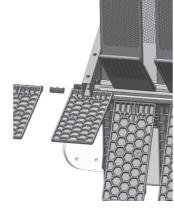
If you are replacing all the slats, do this one row at a time. To do this, you have to keep turning the roller at a slow speed to allow access to all rows.
