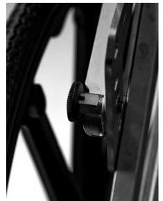
Adjust the handle (1) of the fruit picker to your height at hip height and fix it again by turning the locking pins until they engage in one of the holes. Make sure that both sides have snapped into place at the same height!
